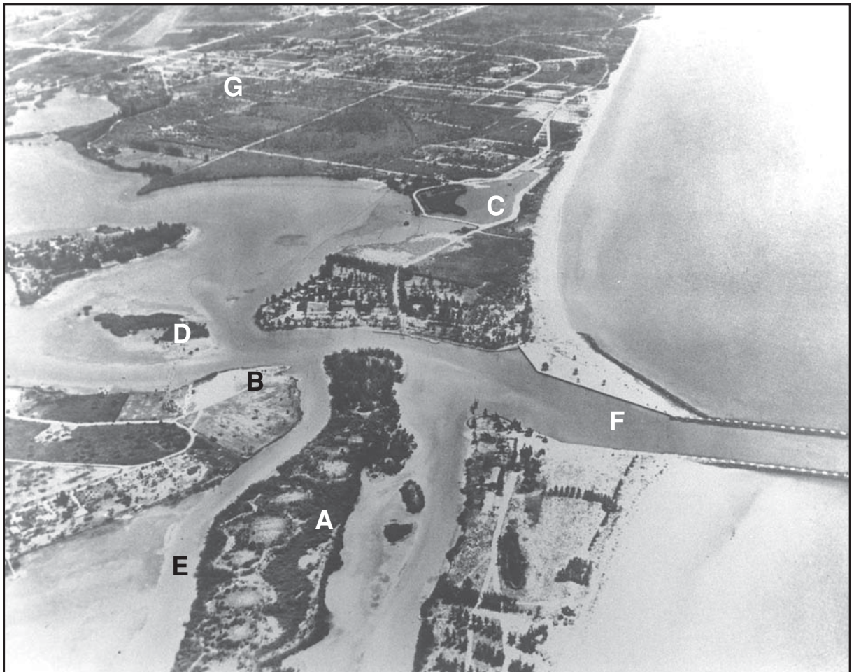
Photo 4. Aerial view south of Venice Inlet, around 1940, showing spoil placement on Turner Key from ICW dredging of original channel
