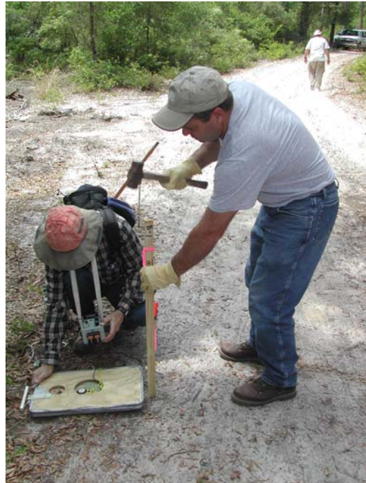
Locating subsurface conduits with radio telemetry and cave divers, Manatee Spring. Wells were installed into three conduits utilizing this technology to better monitor water quality and discharge at Manatee Spring. Photo by: Harley Means, FGS
