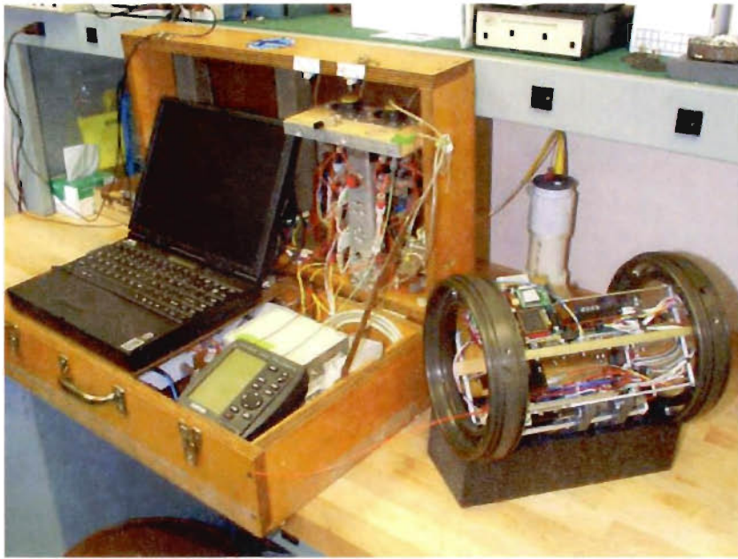
Figure 1 Prototype shipboard Optically-based Phytoplankton Discriminator (OPD) (left). Miniaturized, reconfigured OPD payload for AUVs (right).
