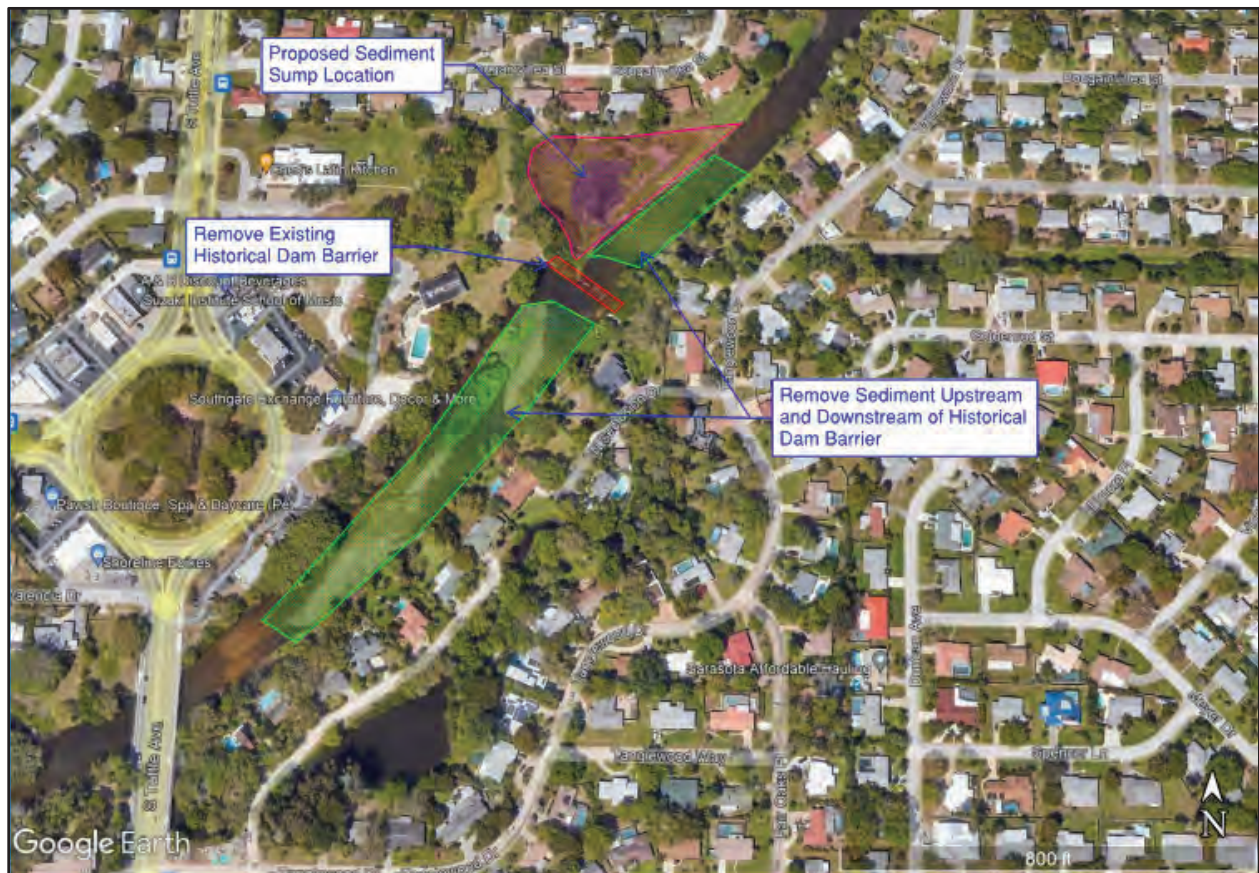
Figure 39 - Tuttle Sediment Removal, Dam Removal and Sediment Sump
