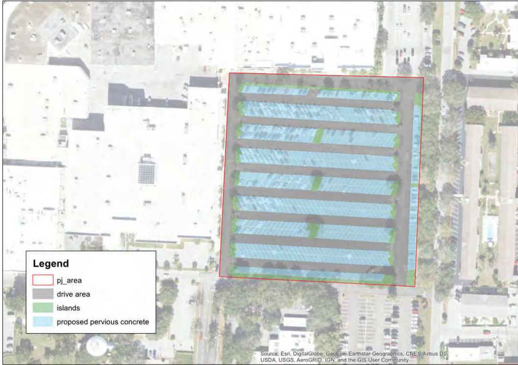
Figure 57 - Westfield Mall Parking Lot Conversion to Pervious Pavement
