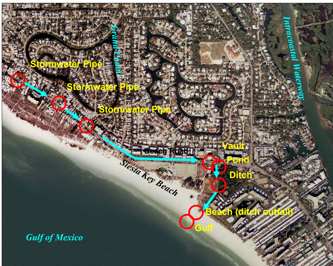
Figure 5. Sampling locations within the stormwater system draining to Siesta Key Beach (light blue arrows indicate general direction of stormwater flow).
