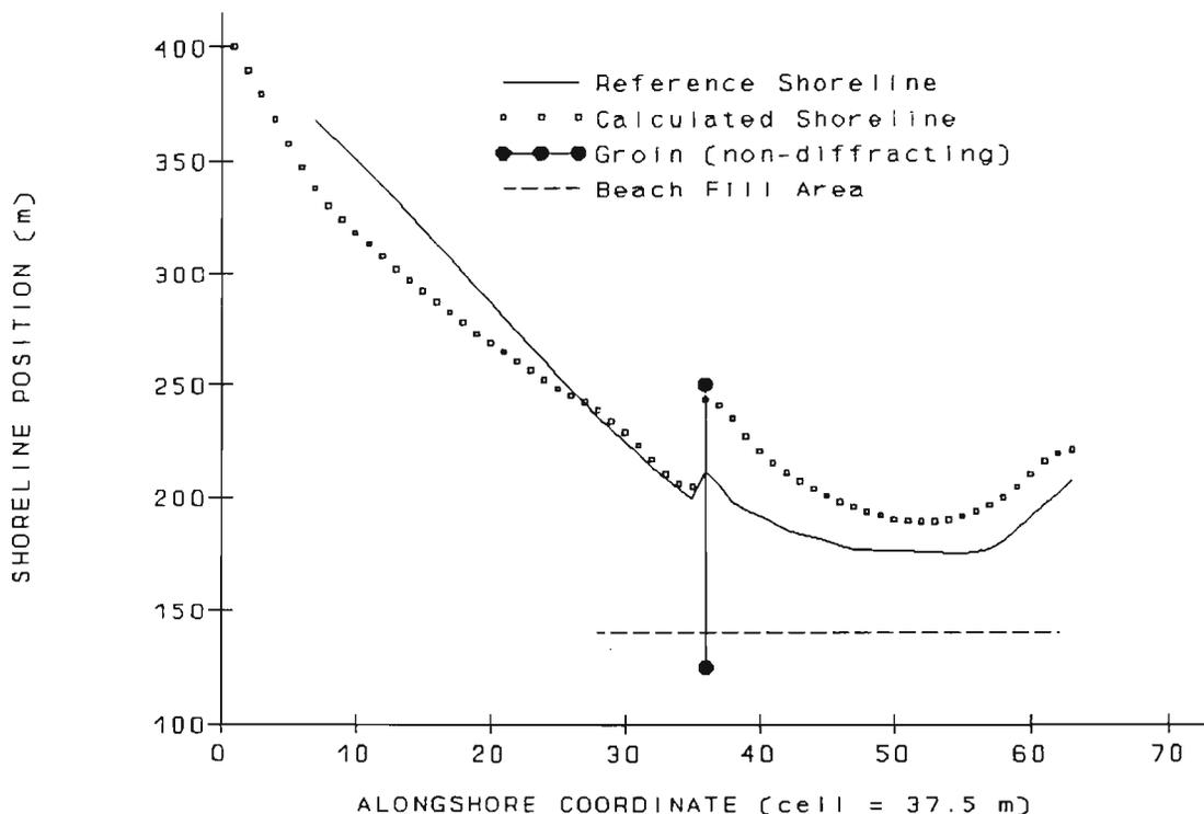
**Figure 11.** Calculated shoreline with groin and fill extended.
