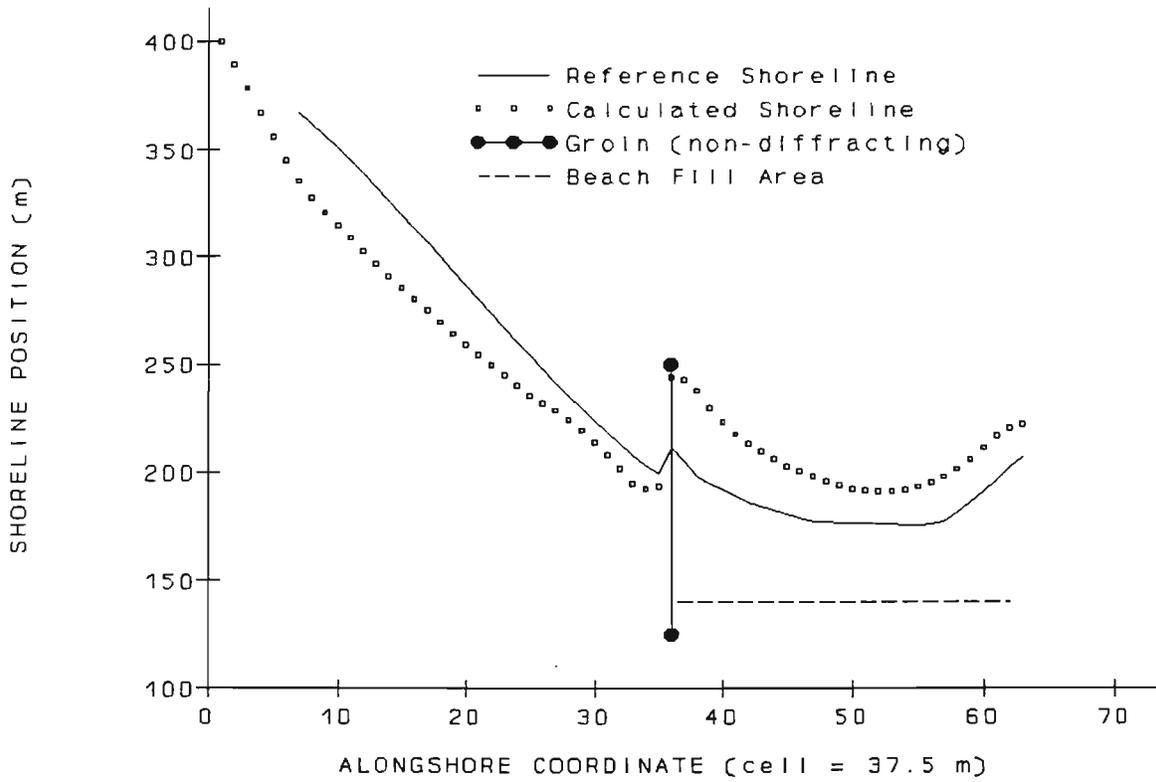
**Figure 10.** Calculated shoreline with an extended groin.
