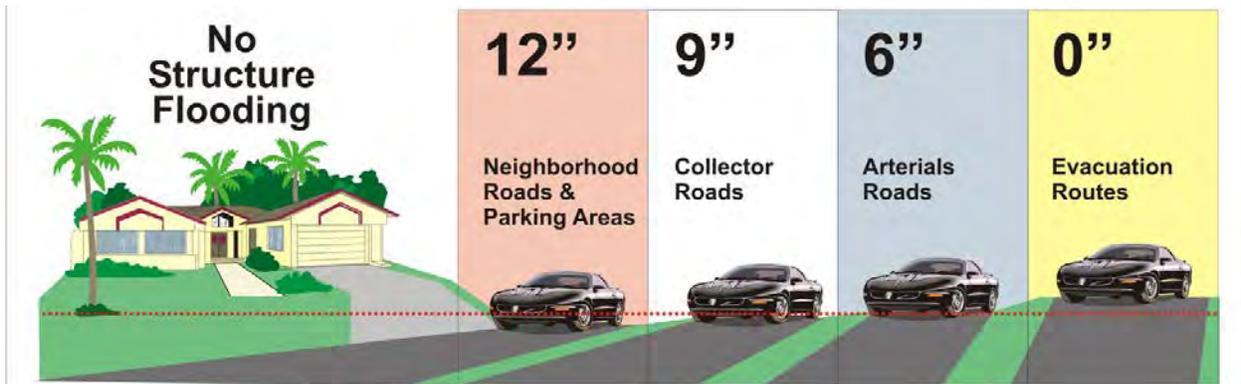
Figure 4-1 Acceptable Flooding for a 100-Year Storm
